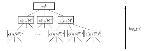
To compute the result of the recurrence, we simply need to add up all the values in the tree. We can do this by adding them up level by level. The top level has value  $cn^k$ , the next level sums to  $ca(n/b)^k$ , the next level sums to  $ca^2(n/b^2)^k$ , and so on. The depth of the tree (the number of levels not including the root) is  $\log_b(n)$ . Therefore, we get a summation of:
